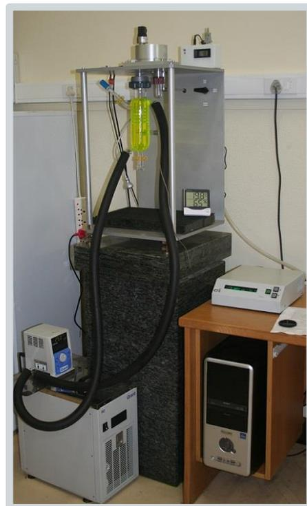
This system, purchased in 2009, consists of a MK2-M5 weigh head with PTFE coating and fixed temperature control, DISBAL control unit, LabWeigh software and accessories pack. Dr Barbour writes his own software for monitoring weight with time, and for sample analysis. They often also use Excel. Reliability and ease of use/implementation are the reasons he gives for choosing to buy CI Precision’s microbalances over others on the market.
