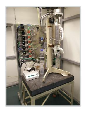
As we integrate reaction and separation, the reaction kinetics and the sorption kinetics are of primary importance to be able to design the reactor. For this reason, most of the studies we perform are on gas/solids reaction kinetics up to 1200°C, multi-cycles stability tests, sorption kinetics etc.
